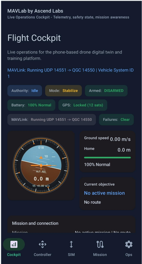
(a) Cockpit — attitude/altitude instrument, ground-speed and home-distance readouts, and armed/mode/battery/GPS/failure cards. The MAVLink status line reports the live endpoint (Running UDP 14551 → QGC 14550 | Vehicle System ID 1).
